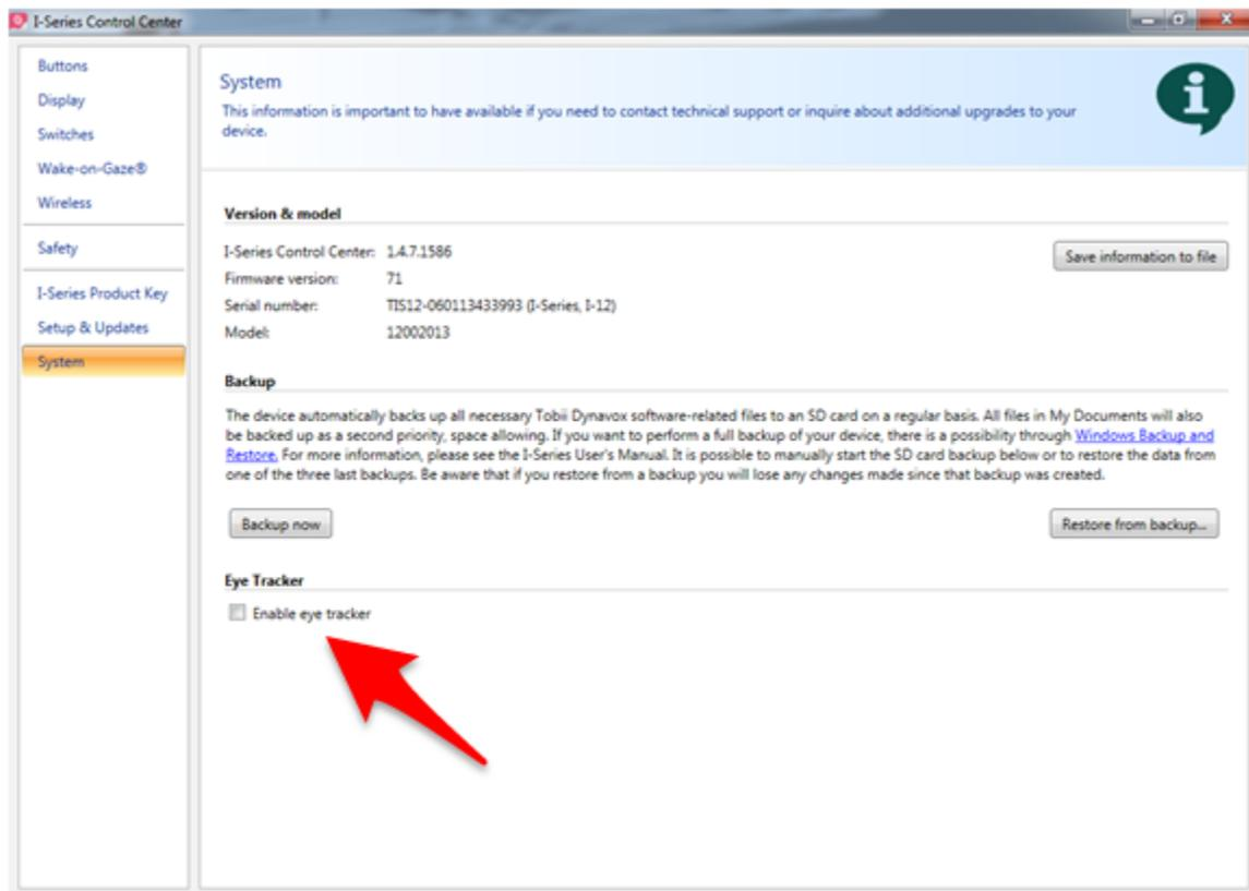
Figure 5 i-Series Control Center with the System settings selected. Un-check the box to disable the eye tracker.
