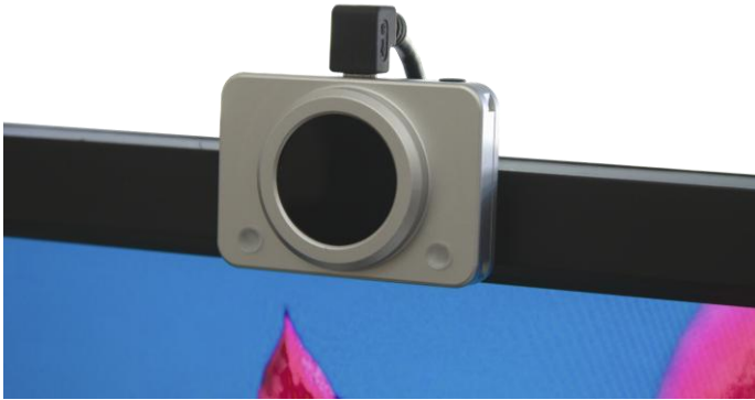
Figure 4: Use the included Dual Lock to attach HeadMouse directly to the monitor bezel.
