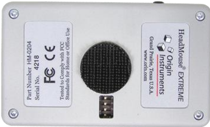
Figure 3: HeadMouse Extreme Rear Panel.
