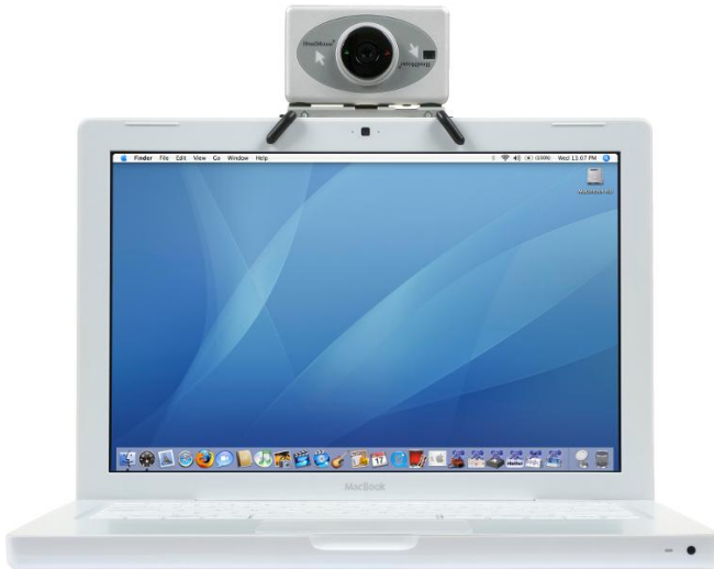
Figure 5: HeadMouse Extreme mounted to a laptop computer
