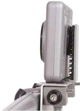
Figure 7: HeadMouse Extreme in Notebook Mounting Bracket (side view)
