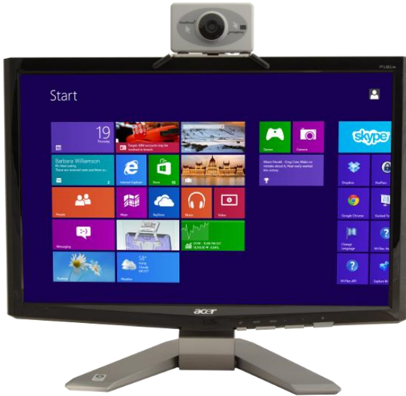
Figure 4: HeadMouse Extreme mounted to a desktop display
