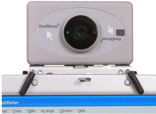
Figure 6: HeadMouse Extreme in Notebook Mounting Bracket
